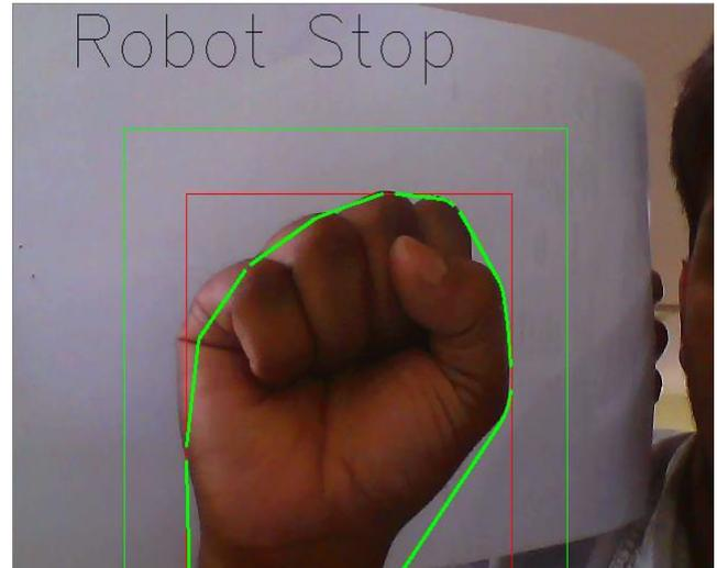
Fig. 5. No dots to stop the robot
