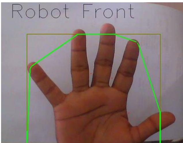
Fig. 4. Five dots to move forward
