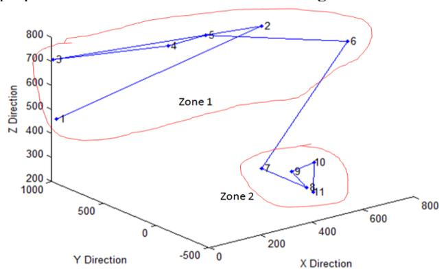
Figure 6. Optimum path of the task locations for zone 1 and zone 2 using TSP-GA.
