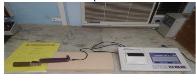
Figure 28. Digital image of composite specimen during surface roughness measurement.
