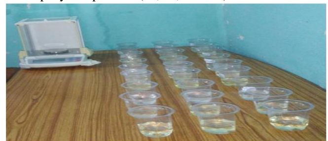
Figure 13. Digital image of the water absorption specimens (micro, macro particle and short fiber composites) immersed in the sea, distilled and tap water.
