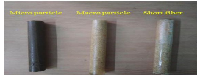
Figure 27. Digital image of the composite rod for micro, macro particle and short fiber reinforced with epoxy composites
