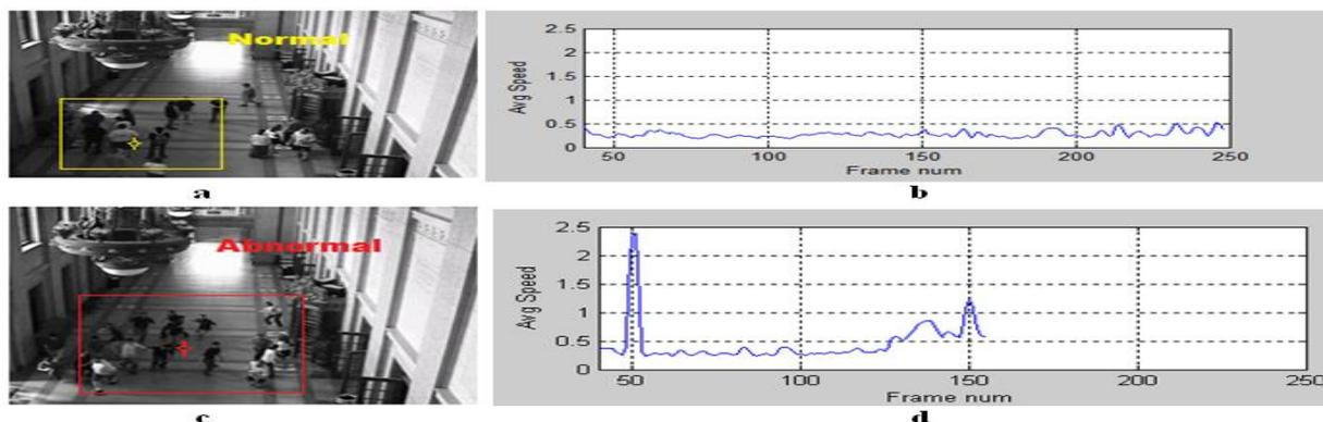
Fig 3. The sample result of the indoor UMN dataset a) Tracking Normal frame b) Speed graph obtained for normal movement in video sequence c) Tracking Abnormal frame d) Speed graph obtained for abnormal movement in video sequence
