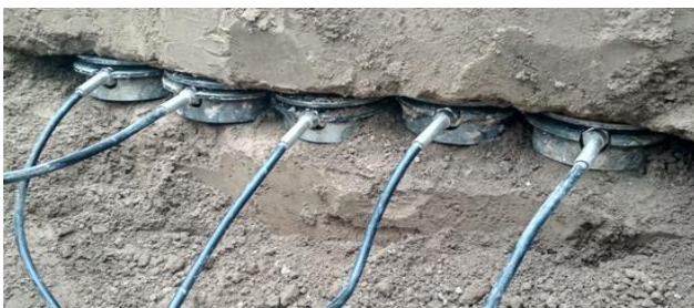
Fig. 3. Installation of sensors in one row across the width of the front tire to the depth of the root layer of the soil
