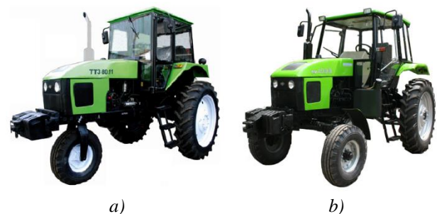
Fig. 1. Tractors TTZ-80.11 with a wheel formula 3K2 (a) and TTZ-1033 with a wheel formula 4K2 (b)
