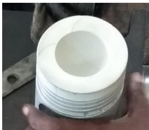
Figure 3. Piston with 200 micron Zirconium Oxide Coating referred as Coated Piston in this paper.
