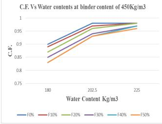
Fig. 7. C.F. Vs Water contents at binder content of 450Kg/m<sup>3</sup>
