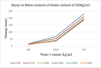
Fig. 4. Slump and Water contents at binder content of 450Kg/m<sup>3</sup>
