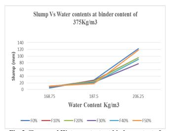
Fig. 3. Slump and Water contents at binder content of  $375 \text{Kg/m}^3$
