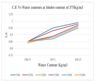
Fig. 6. C.F. Vs Water contents at binder content of 375 Kg/m<sup>3</sup>
