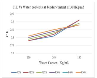
Fig. 5. C.F. Vs Water contents at binder content of 300 Kg/m<sup>3</sup>
