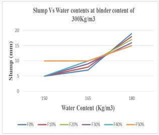
Fig. 2. Slump and Water contents at binder content of  $300 \text{Kg/m}^3$
