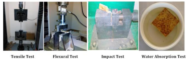
Figure 3 Experimental Setup for Mechanical Characteristics and Water absorption test.
