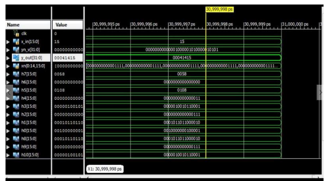
Fig.7.Simulation result of 15 tap FrFT based FIR LPF with binary representation of coefficients.
