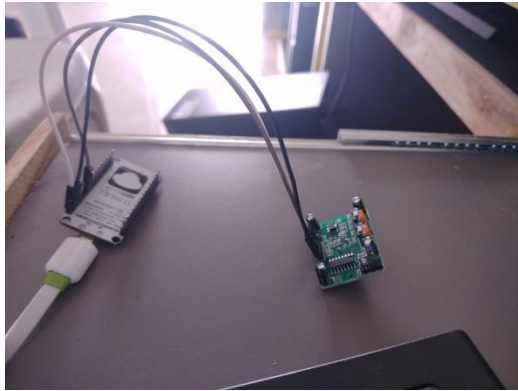
Fig 9: Connections with PIR Sensor
