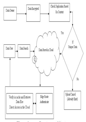
Figure 1: overall system architecture
