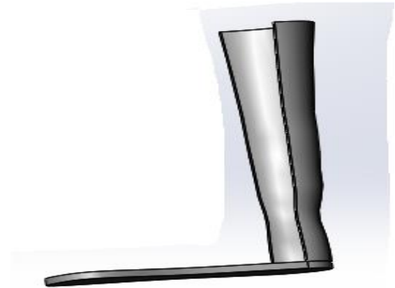
Figure 3. Model of the AFO obtained in solidworks©
