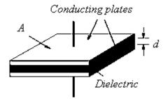
Figure 3 Parallel Plate Capacitor
