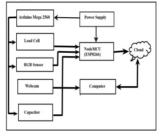
Figure 1 Block Diagram for Non-Invasive Fruit Analyser\_1.7
