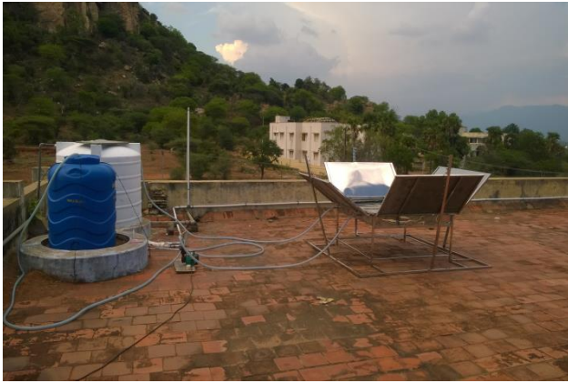
Fig.1.1 (a) Experimental setup of Bin model solar instant water heater for performance analysis
