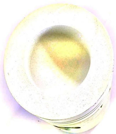
Figure 3: Zirconia Coated Piston – Crown Only.
