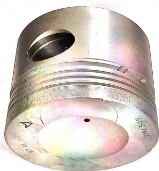
Figure 2: Normal Cast Aluminium Alloy Piston
