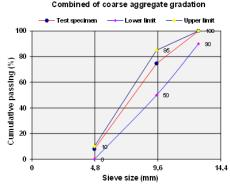
Fig. 7. Gradation curve for combined coarse aggregate
