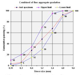
Fig. 6. Gradation curve for combined fine aggregate
