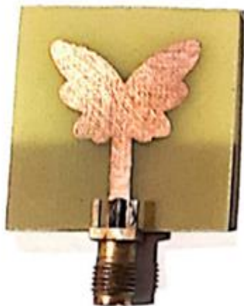
Fig 6.1: Fabricated design of four arm butterfly shaped antenna
