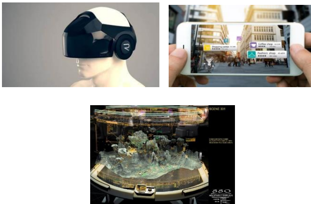
Figure 4: Head Mounted Display, Hand-held Display and Projected Based
