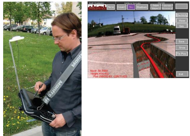
Figure 18: AR with GPS(left). virtual excavation (right). Courtesy of Gerhard Schall [21]
