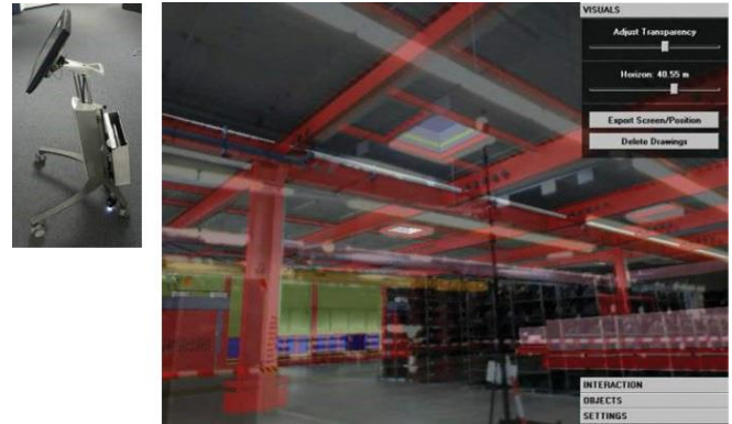
Figure 17: The touchscreen display (left), which can be used for discrepancy analysis directly on the factory floor (right). Courtesy of Ralph Schönfelder. [21]
