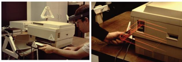
Figure 12: HMD on printer maintenance. Courtesy of Steve Feiner, Blair MacIntyre, and Doreé Seligmann, Columbia University.[21]
