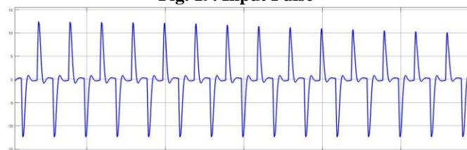
Fig. 20. Output at the inverter
