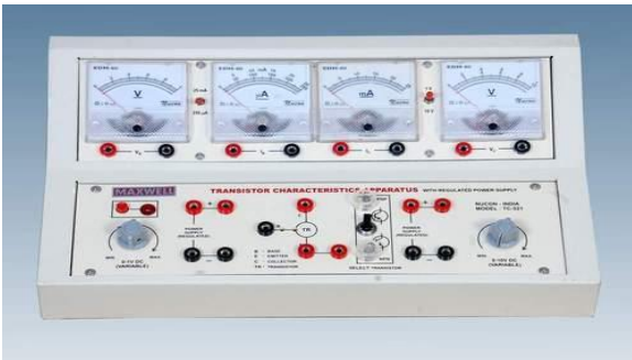
Figure 2: A device which measure input and transfer characteristics of both NPN and PNP transistors
