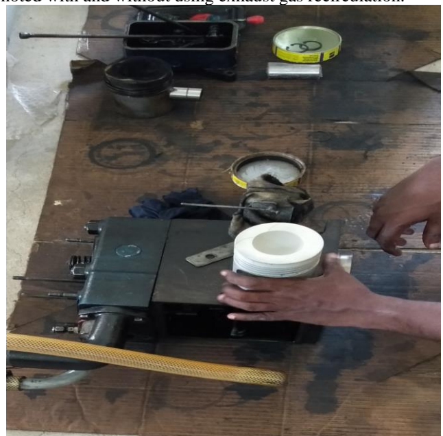
Figure 1: Coated Piston – Zirconium Oxide – Thermal Barrier Coating.
