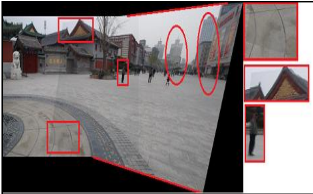
Fig. 4 Stitching Result using APAP method on Temple dataset
