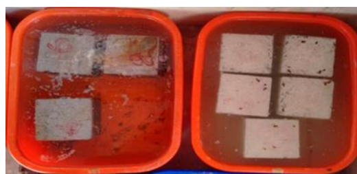
Fig5 Specimens immersed in diluted Hcl and H 2 SO 4
