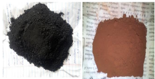
Fig. 4 Carbon, Iron oxide samples before surface grinding
