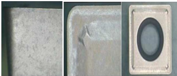
Fig.2. optical microscope images of (a) Flank surface (b) Rake face (c) coated carbide insert
