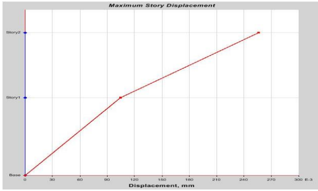
Fig. 15. Maximum Storey Displacement for Frame 3 in Storey 2 is 255 \times 10^{-3} mm
