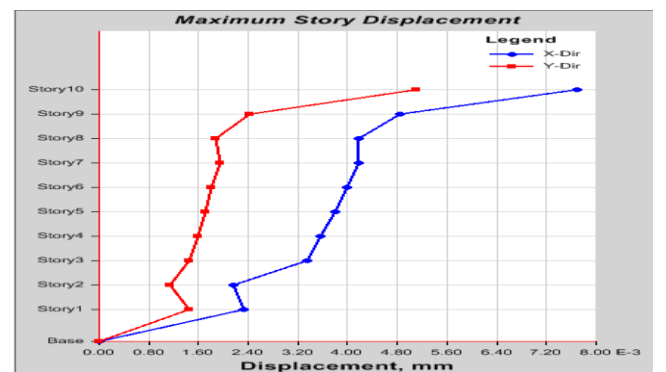
Fig. 22. Maximum Storey Displacement for Model 4 in Storey 10 is 7.8 \times 10^{-3} mm (X -Direction)
