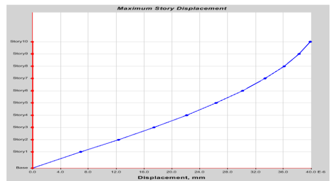
Fig. 20. Maximum Storey Displacement for Model 2 in 10 th Storey is 40 \times 10^{-6} mm
