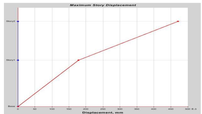
Fig. 13. Maximum Storey Displacement for Frame 1 in Storey 2 is 470 \times 10^{-3} mm
