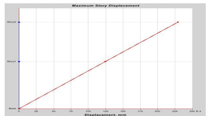
Fig. 14. Maximum Storey Displacement for Frame 2 in Storey 2 is 230 \times 10^{-3} mm
