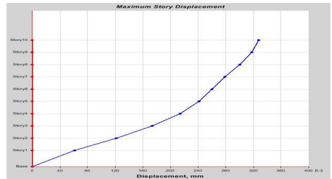
Fig. 19. Maximum Storey Displacement for Model 1 in 10 th Storey is 325 \times 10^{-3} mm
