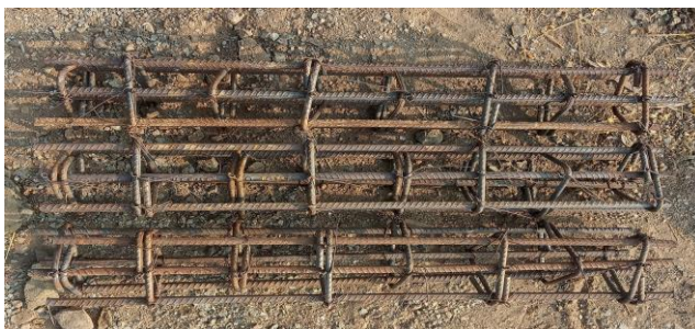
Fig.8 Triangular shape stirrups @ 90 mm c/c spacing
