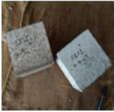
Fig.10. Concrete after Curing
