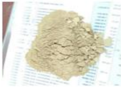
Fig.6. 50g Fine passed through 0.075 mm sieve
