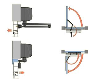
Fig. 1.Openingmechanism of a swing automatic door.
