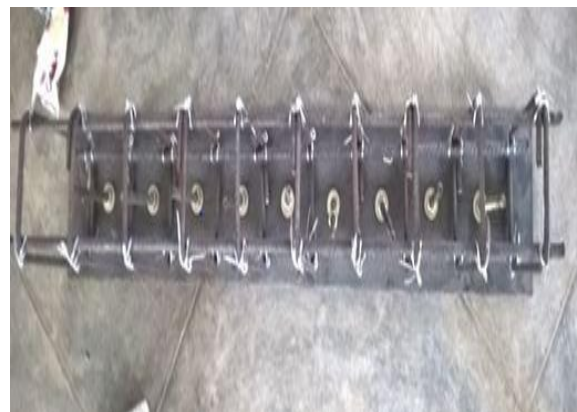
Fig. 4: Single row bolt arrangements with steel plate having reinforcement cage
