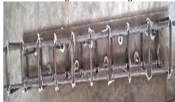
Fig. 5: Stagger row bolt arrangements with steel plate having reinforcement cage
