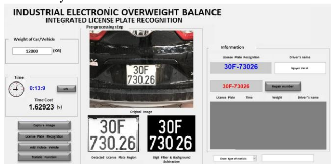
Fig. 13. Interface of License Plate Recognition Integration Application
