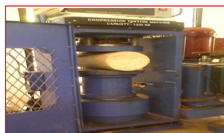
(b) Split tensile setup
