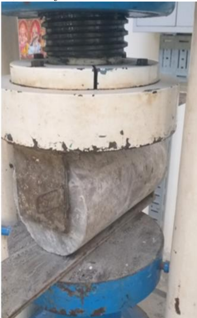
Fig. 3. Split Tensile test on Foam concrete specimen
