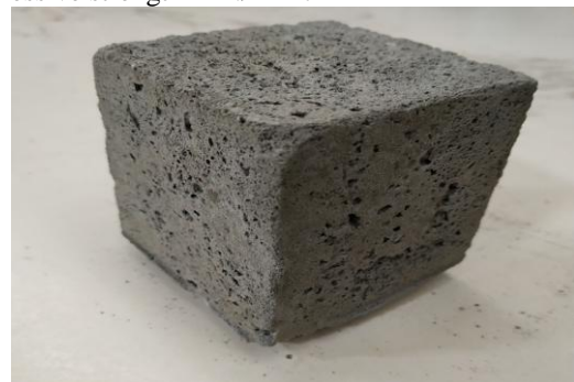
Fig. 2. Foam concrete specimen before testing
