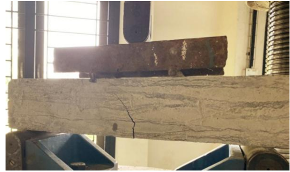
Fig. 4. Flexural Strength test on Foam concrete specimen
