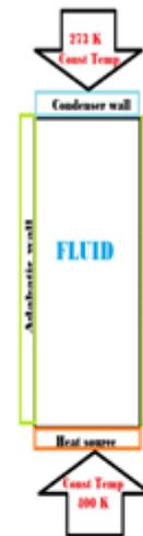
**Figure 1: Line diagram with specified boundary conditions**
