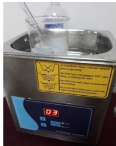
Figure.5. Ultra sonication process of MWCNT's and SiO
