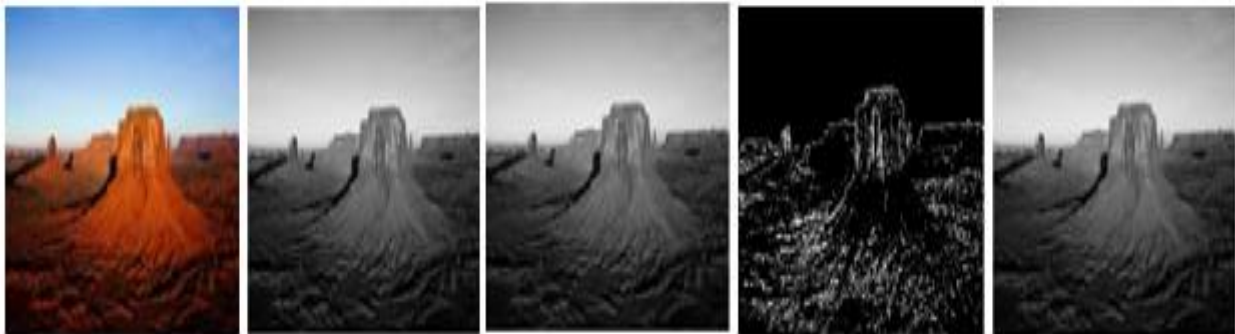
Fig.3 (a) Input Image (b) Convert into gray(c) Enhanced Image (d) Edge detection (e) Enhanced after fuzzy
