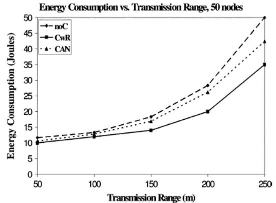
**Fig. 4. Effect of transmission power on consumption**
