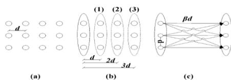
**Fig.3. Grid topology. (a) Placement of nodes. (b) formation of clusters. (c) Intra-versus inter-cluster distances.**
