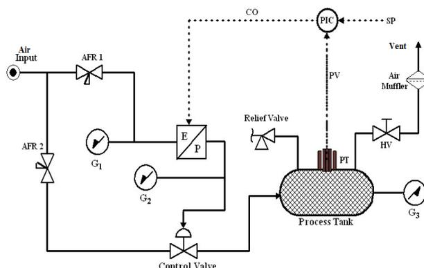
Fig. 1. Schematic view of Air Pressure System (APS)
