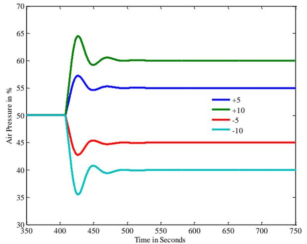
**Fig. 11. Set point tracking at 50 % pressure using SGC controller**
