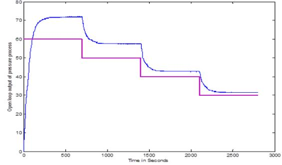
Fig. 3. Open loop responses (10% Negative step changes) - APS
