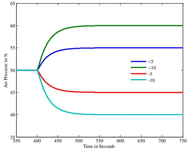
**Fig. 10. Set point tracking at 50 % pressure using FGC controller**
