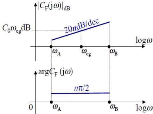
Fig. 5. Bode plot of FGC controller
