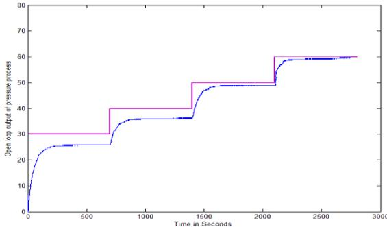
Fig. 2. Open loop responses (10% Positive step changes) – APS
