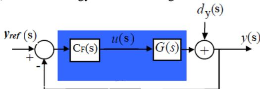
y<sub>ref</sub>(s) - input reference signal, d<sub>y</sub>(s) – Process output disturbance, u(s) - controller output, C<sub>F</sub>(s) – First generation CRONE controller, G(s) - Process transfer function, y(s) - plant output
