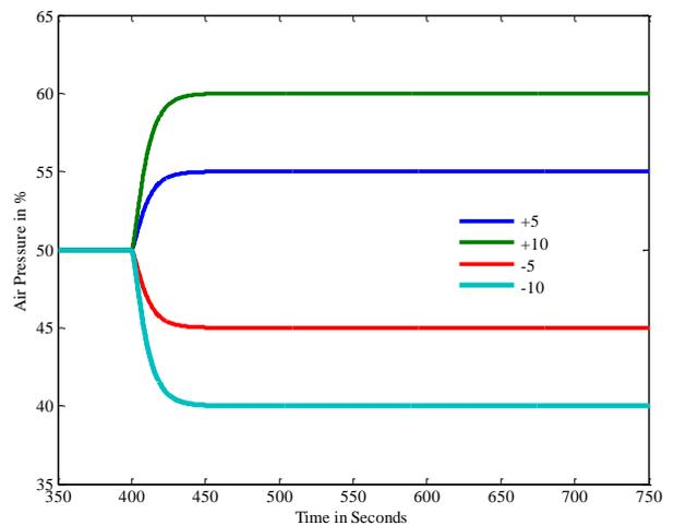
**Fig. 12. Set point tracking at 50 % pressure using TGC controller**
