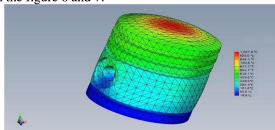
**Figure 6.temperature distribution on a conventional piston made of cast aluminium alloy**
