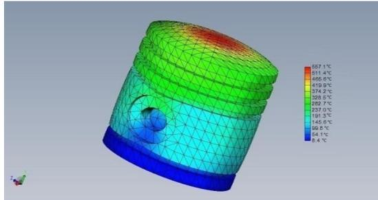
Figure 7. temperature distribution on a magnesium stabilized zirconia piston
