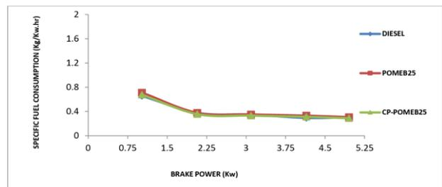
Figure 1. variation of specific fuel consumption with brake power
