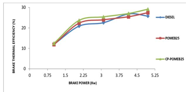
Figure 2. variation of brake thermal efficiency with brake power
