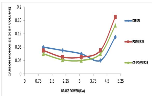
**Figure 3.variation of carbon monoxide emission with brake power**
