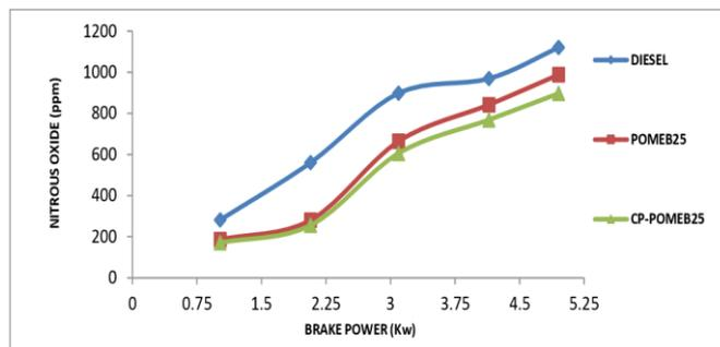
**Figure 5.variation of nitrous oxide emission with brake power**
