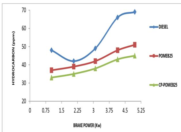
**Figure 4.variation of hydrocarbon emission with brake power**
