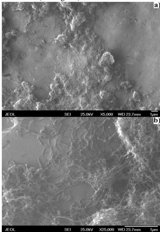
**Fig. 1. Electronic micrographs at different magnifications of initial multi-walled carbon nanotubes.**
