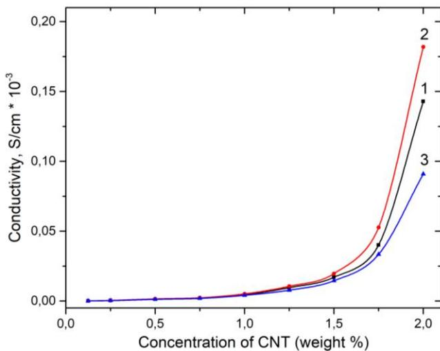
**Fig. 4. Concentration dependence of the electrical conductivity of composite material (1-initial MWNTs; 2-MWNTs treated in isopropyl alcohol; 3- MWNTs treated in nitric acid).**
