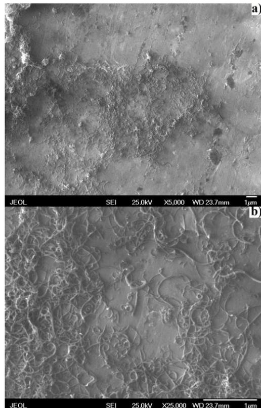
**Fig. 3. Electronic micrographs at different magnifications of multi-walled carbon nanotubes treated in nitric acid.**
