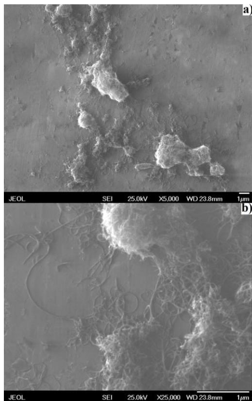
**Fig. 2. Electronic micrographs at different magnifications of multi-walled carbon nanotubes treated in isopropyl alcohol.**
