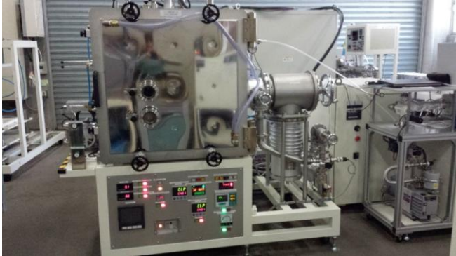
Fig. 2 the induction furnace used for carbo-thermal reduction
