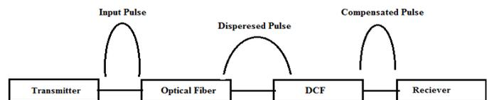
**Fig 1. Block Diagram of DCF Compensated Optical Link** Finally equation 1, 2, 3 can be combined to determine total losses as given in equation 4.
