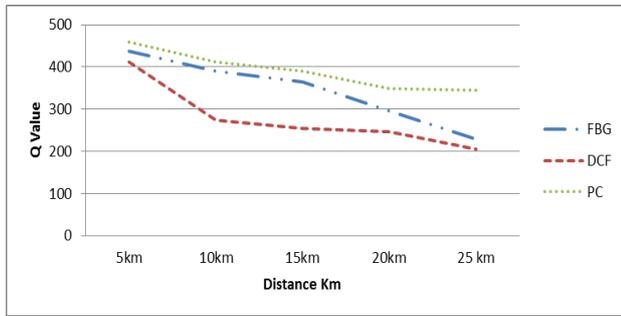
Fig. 3.2 Q value versus Distance Km for Channel 2
