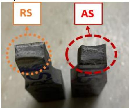
Fig. 13. Specimen -2 fracture occurred at 710 rpm
