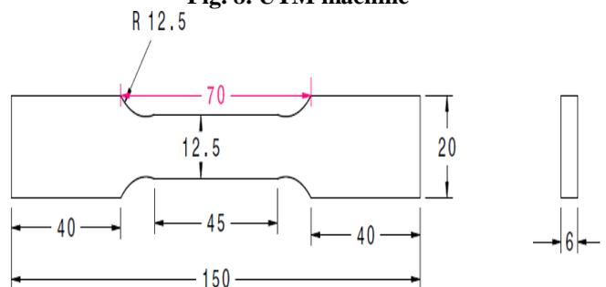
**Fig. 9. Design of tensile specimen as per the ASTM E8M-04 standard**
