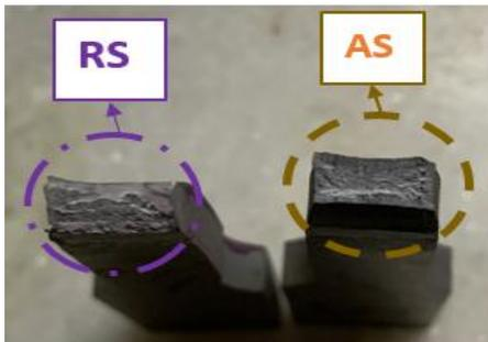
Fig. 12. Specimen -1 fracture occurred at 710 rpm
