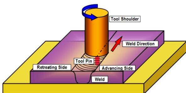
Fig. 1. FSW of butt joints [3]
