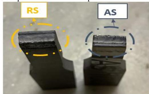
Fig. 14. Specimen -1 fracture occurred at 900 rpm
