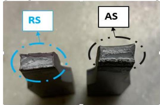
Fig. 15. Specimen -2 fracture occurred at 900 rpm
