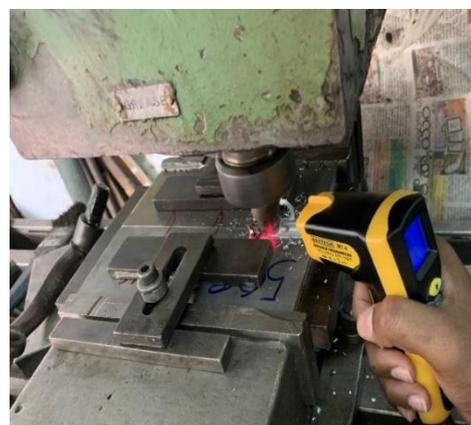
Fig. 3. Infrared Thermometer employed for measuring temperatures across the weldments
