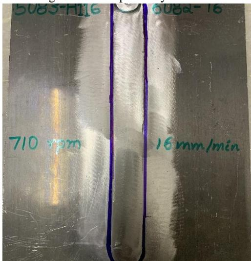
**Fig. 6. Weldment fabricated at 710 rpm**
