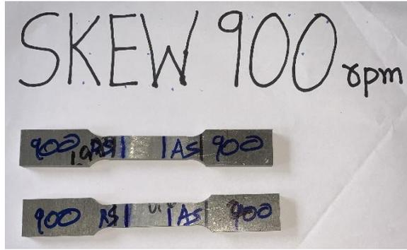
Fig. 11. Dissimilar Aluminium Alloys Tensile specimens at 900 rpm
