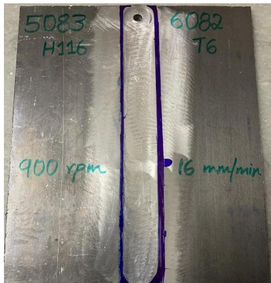
**Fig. 7. Weldment fabricated at 900 rpm**
