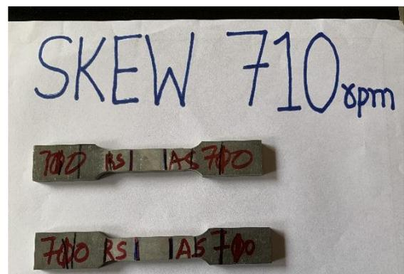
**Fig. 10. Dissimilar Aluminium Alloys Tensile specimens at 710 rpm**
