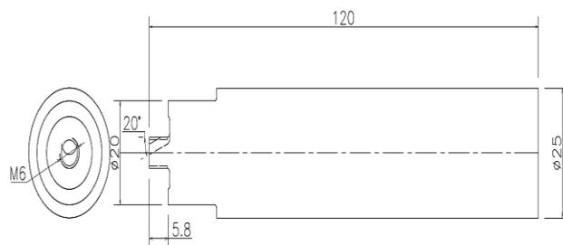
Fig. 4. Design of skew tool pin profile
