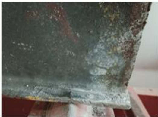
Fig.9 Little buckling of flange at support
