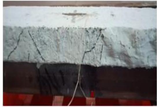
Fig.10 Minor cracks developed in slab
