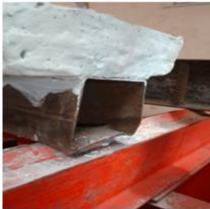
Fig.14 Buckling of hollow section at support
