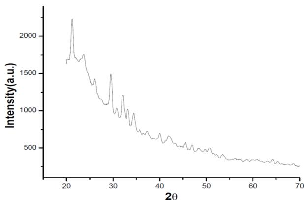
**Fig.9: XRD of terpolymeric nanocomposite (with silver nanoparticles)**
