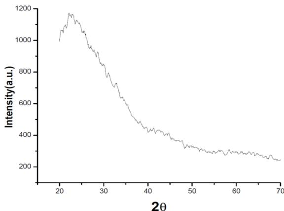
**Fig.8: XRD of terpolymeric composite (without silver nanoparticles)**
