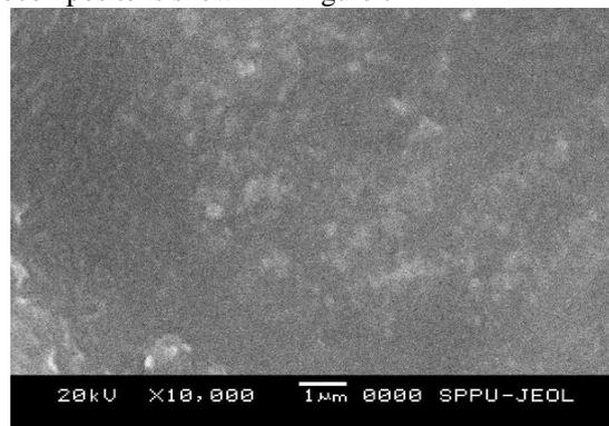
Fig.6 SEM image of terpolymeric composite (without silver nanoparticle)
