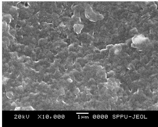
**Fig.7 SEM image of terpolymeric composite with silver nanoparticle**
