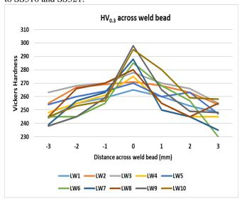
Fig. 5: Vickers Hardness across weld bead
