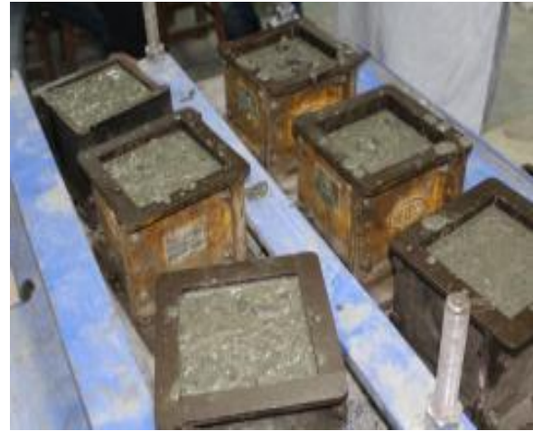
Fig. 3: Casting of Concrete Specimens in the laboratory
