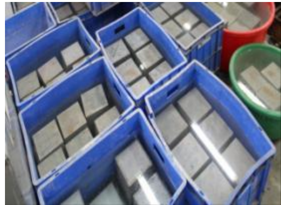
Fig. 4: Curing of Concrete Specimens
