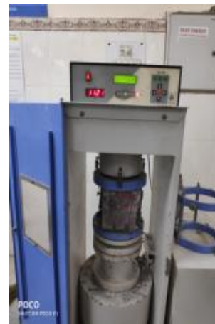
Fig. 5: Testing of Concrete Specimens
