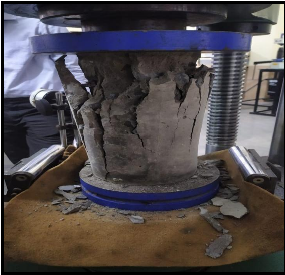
Fig. 11: Shear failure in Unconfined Specimen
