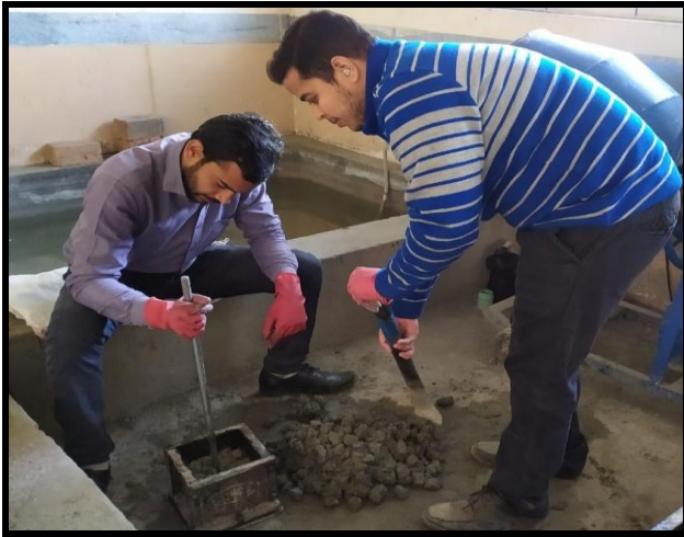
Fig. 3: Casting of Cube
