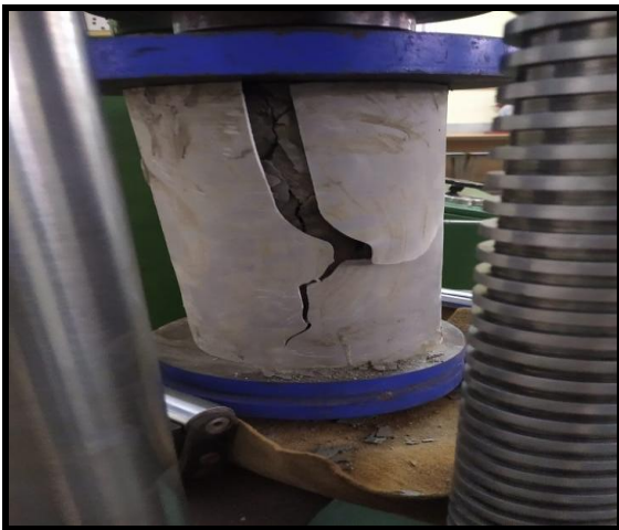
Fig. 12: Shear failure in Confined Specimen of 2.5 mm Thickness
