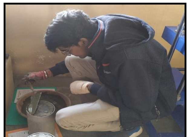
Fig. 7: Application of Cement Slurry
