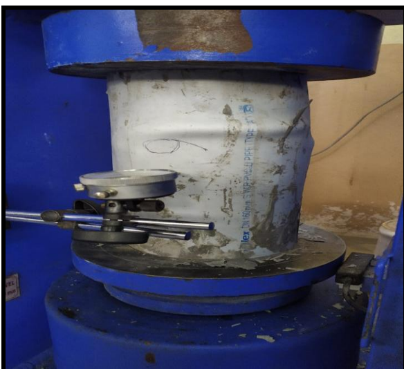
Fig. 13: Drum Type failure in Confined Specimen of 3.5 mm Thickness
