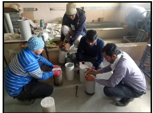
Fig. 6: Confinement of column using U-PVC Pipe
