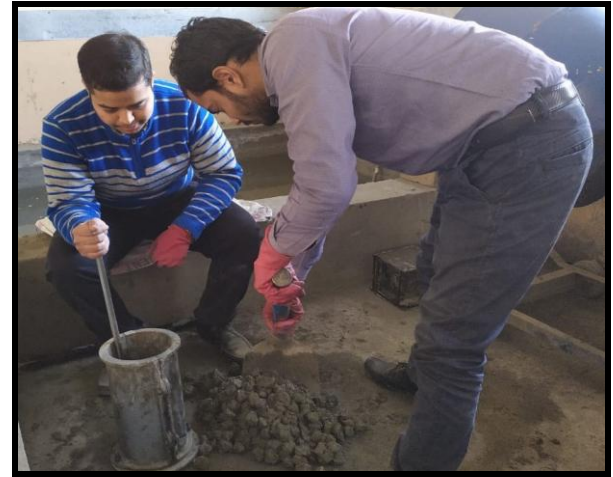
Fig. 5: Casting of Cylinder
