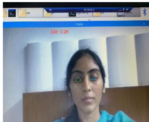
Fig 11. Decrease in value of eye aspect ratio when eyes are half closed.
