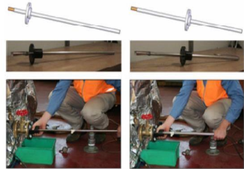
Fig.7. Insertion of antenna
